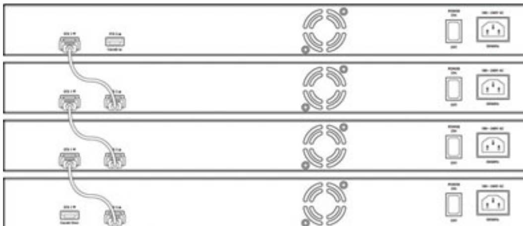
Figure 4-118: Chain Stack topology
