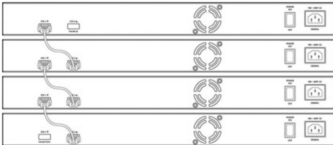
Figure 2-16: Chain Stack topology
