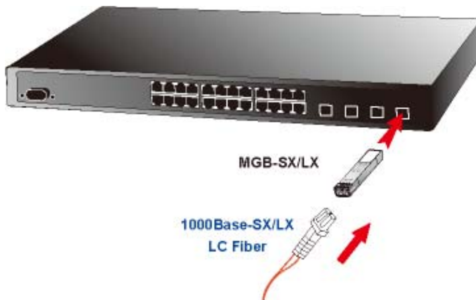
Figure 2-14: Plugging-in the SFP transceiver
