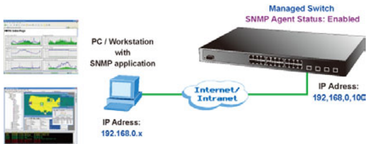
Figure 3-5: SNMP management setup
