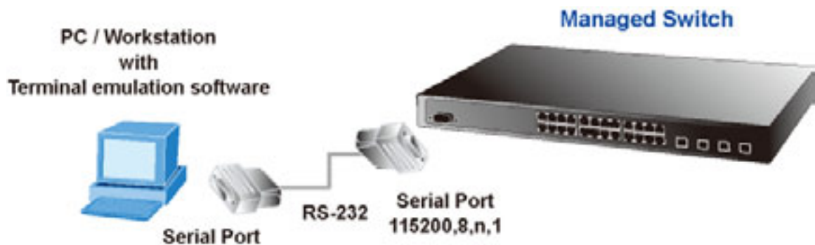
Figure 3-1: Console management Setup
