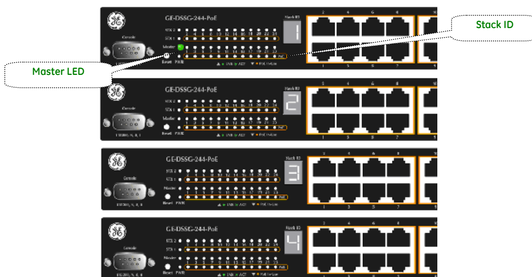
Figure 2-19: Stack Master with "Master" LED lit
