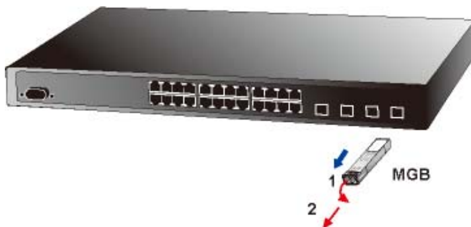
Figure 2-15: Pulling out the SFP transceiver
