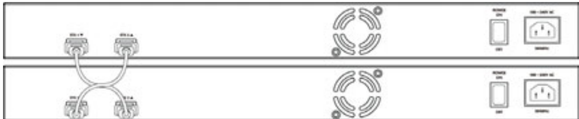
Figure 4-120: Back to back Stack topology
