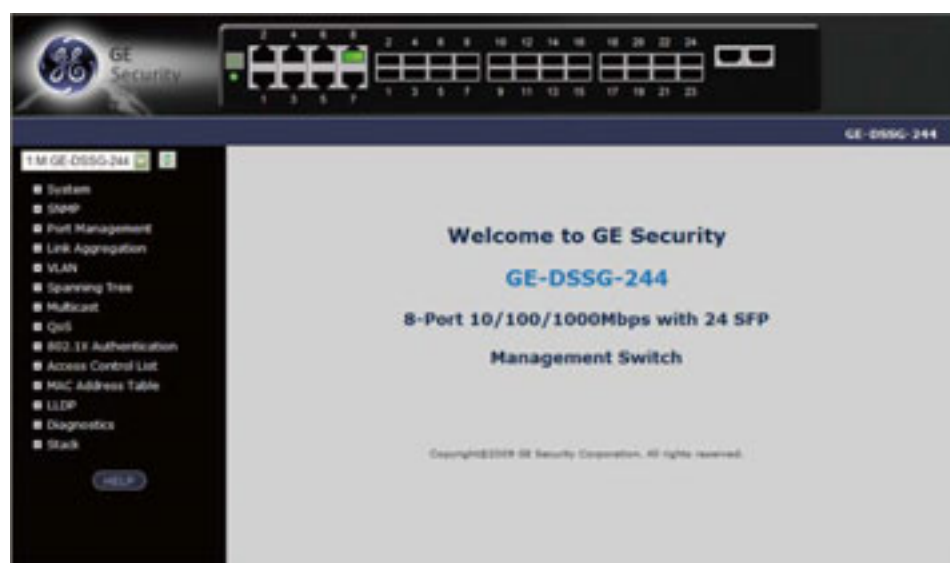
Figure 3-4: Web main screen of Managed Switch
