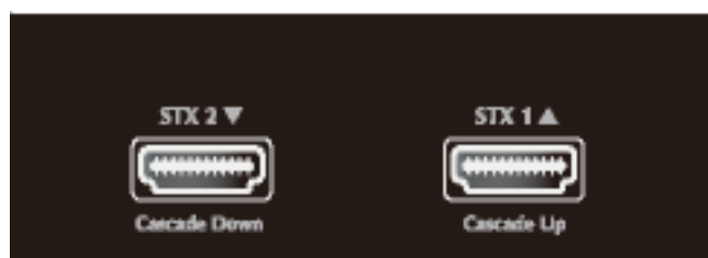
Figure 2-10: GE-DSSG-244 Stack Ports
