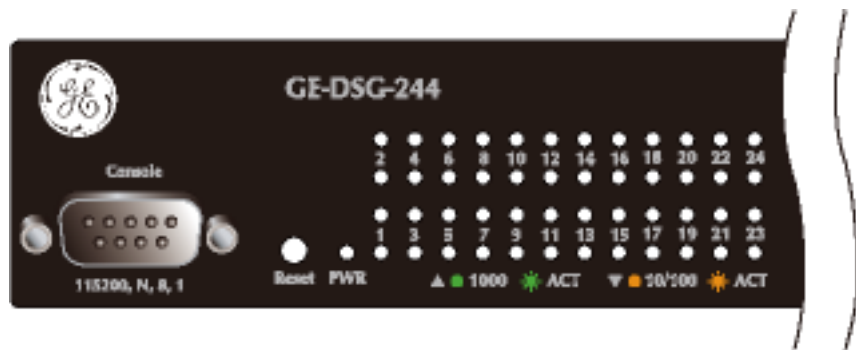
Figure 2-4: GE-DSG-244 LED indication
